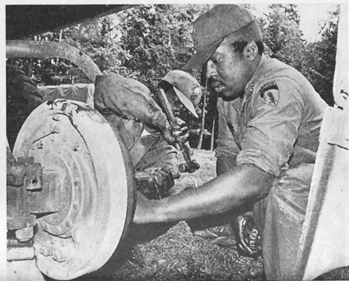
PACKING THE BEARINGS on a deuce-and-a-half is a simple job in Berlin. When 2-6 mechanics are in the field it is complicated by the environmental conditions varying from sleet and rain to dust. PFC Billy Williams, left, and PFC Barry Queener get the job done during the MTA at Hohenfels, FRG. (Photo by Gary L. Swinton)
